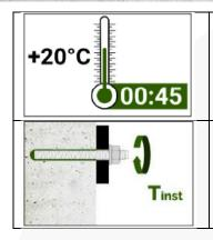
10. Allow the adhesive to cure to the specified time prior to applying any load or torque. Do not move or load the anchor until it is fully cured.
